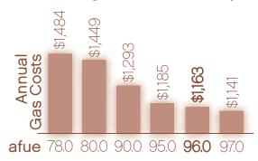
The Infinity® 96 gas furnace offers plenty of potential for annual savings with outstanding gas efficiency. Compared to today's minimum efficiency models, the Infinity 96 can deliver estimated savings of about \$286 annually on your gas costs.† If you are replacing an older furnace, you can save even more. Variable-speed blower and inducer motors contribute electrical savings as well to complete the utility savings story.
